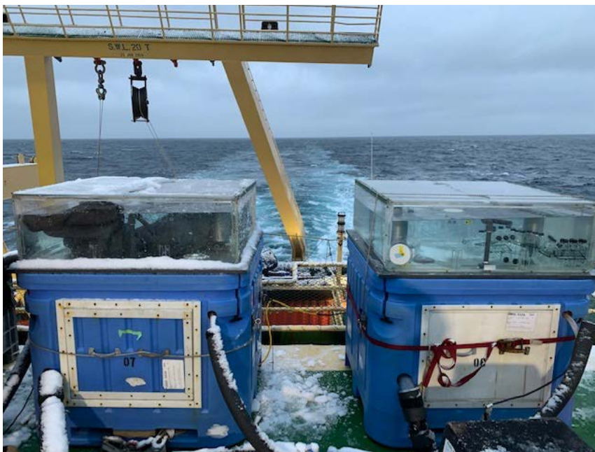
Figure 4. Incubation tanks on the Helo deck of the NBP used for the 24-hour outdoor light incubation experiment.
